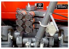
**Improved Hydraulics** The M5L has 2 standard rear remote valves. It now offers 2 self-cancelling detent valves.
