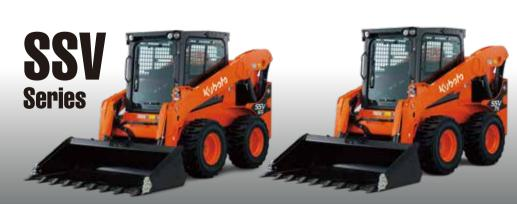
**SSV65** Rated Operating Capacity @ 50% of Tipping Load: 1,950 lbs. (885 kg) Operating Weight: Open CAB 7,099 lbs. (3,220 kg) Closed CAB 7,319 lbs. (3,320 kg) Engine Horsepower: 64.0 (47.7 kW) / 2,700 rpm
