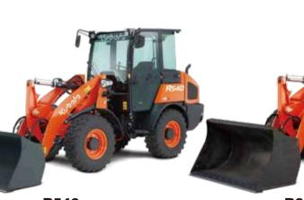
**R540** Operating Weight: CANOPY/CAB 9,888 lbs. (4,485 kg) / 10,285 lbs. (4,665 kg) Bucket Capacity: 0.85 cu.yd. (0.65 m³) Horsepower: 50.9 (38.0 kW) / 2,400 rpm
