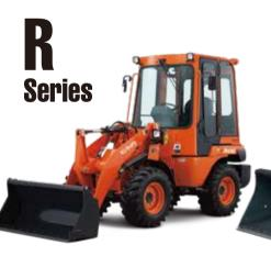
**R430** Operating Weight: CANOPY/CAB 7,758 lbs. (3,519 kg) / 8,232 lbs. (3,734 kg) Bucket Capacity: 0.5 cu.yd. (0.38 m³) Horsepower: 47.6 (35.5 kW) / 2,600 rpm
