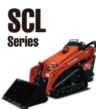
**SCL1000** Rated Operating Capacity @ 35% of Tipping Load: 1,000 lbs. (453 kg)
