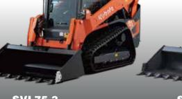
**SVL75-3** Rated Operating Capacity @ 35% of Tipping Load: 2,490 lbs. (1,129 kg) Operating Weight: Open CAB 9,190 lbs. (4,169 kg) Closed CAB 9,420 lbs. (4,273 kg) Engine Horsepower: 74.3 (55.4 kW) / 2,400 rpm
