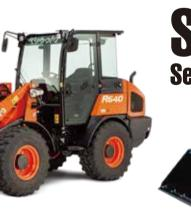
**R640** Operating Weight: CANOPY/CAB 11,177 lbs. (5,070 kg) / 11,563 lbs. (5,245 kg) Bucket Capacity: 0.94 cu.yd. (0.72 m³) Horsepower: 64.3 (48.0 kW) / 2,400 rpm
