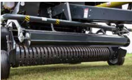
Kubota BV5160-BV5200 with 86" pick-up and roller wind guard.
