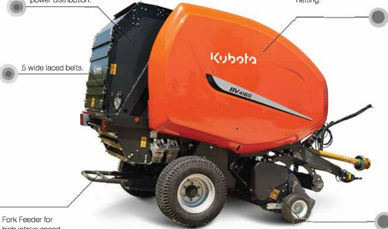
Fork Feeder for high intake speed.
