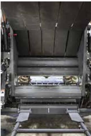
A combination of 5 belts and front rollers provides dense bales with an adjustable core and an easy bale start.
