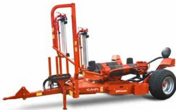
Extra counter weights can be fitted on the left hand side of the machine to ensure full stability also for the heavy bales.
