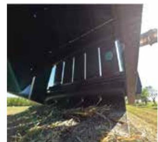
All balers come standard with Silage Scrapers meant for scraping build up of a wet or stringy crop around the rollers. This feature allows for use in dry or wet hay.
