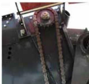
Main bale chamber drive is heavy duty 1 1/4" pitch chain.
