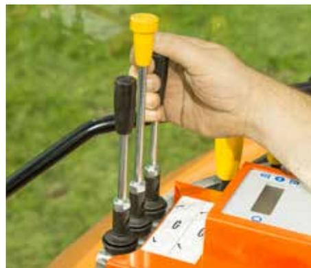
**Mechanical cable control (WR1400M)**
